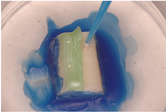
Figure 2 - Desensitizing agent application over the test surface (non-protected)
